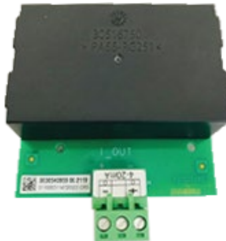
Figure 1-2: Analog Output Option Board for IND500x
