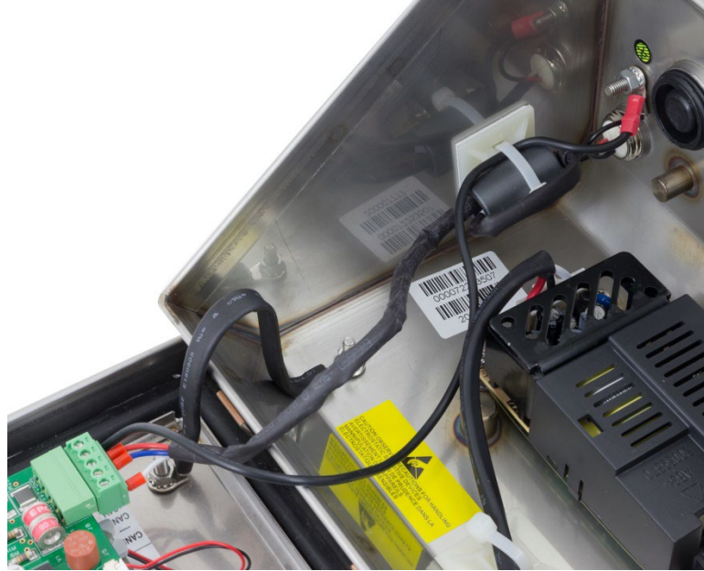
Figure 2-56: PowerDeck Connector Installed in the IND246 POWERCELL
