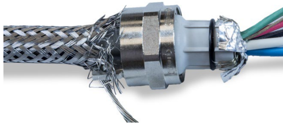
Figure 2-44: Inner Braided Shield Wires and Foil Trimmed to Length and Folded Back Over Grommet
