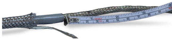
Figure 2-36: Marking the Inner Braided Shield
