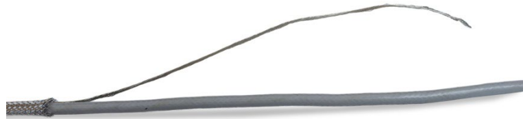
Figure 2-31: Exterior Braided Armor Trimmed Back
