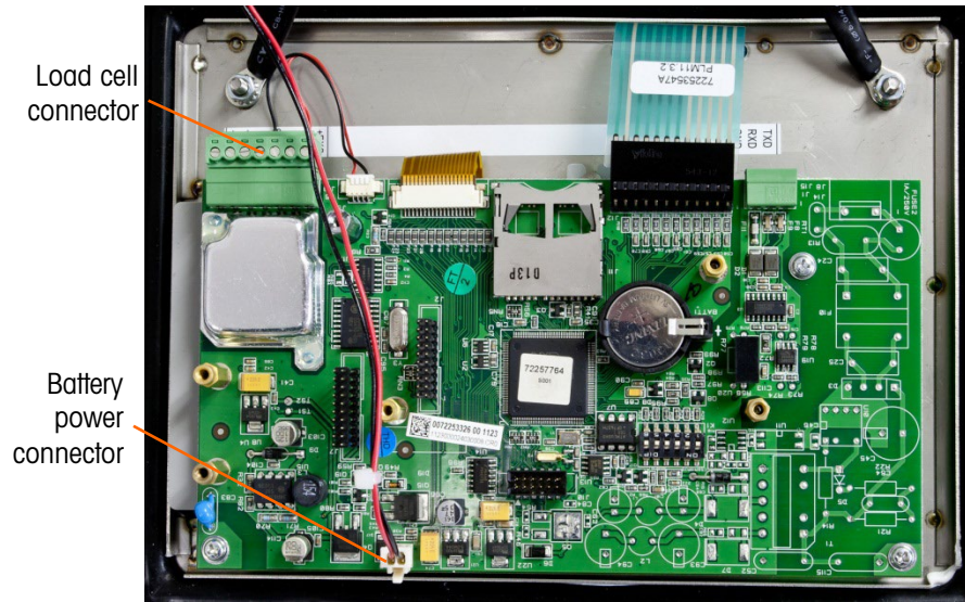
Figure 2-20: IND246 Main Board Connections, Battery-Powered Model
