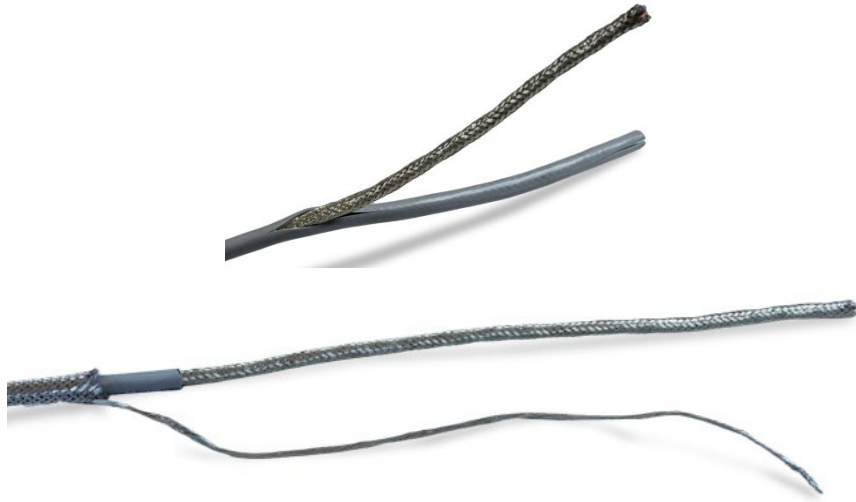
Figure 2-35: Peeling the Cable Jacket away from the Inner Braided Shield
