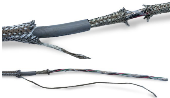
Figure 2-37: Removing the Inner Braided Shield
