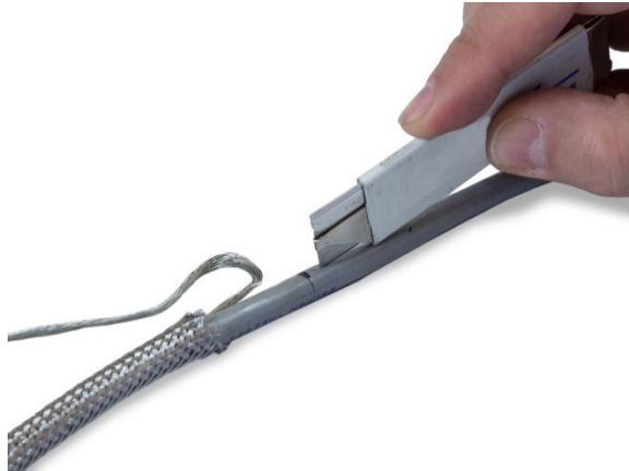
Figure 2-34: Cutting Along the Cable Jacket
