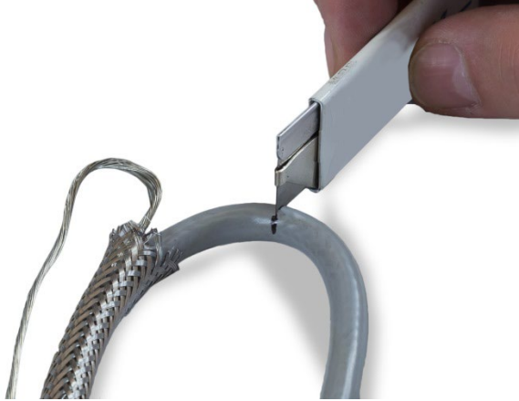
Figure 2-33: Cutting Around Cable Jacket
