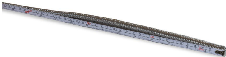
Figure 2-29: Measuring the Exterior Braided Armor Before Cutting
