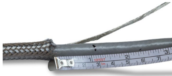
Figure 2-32: Marking the Cable Jacket
