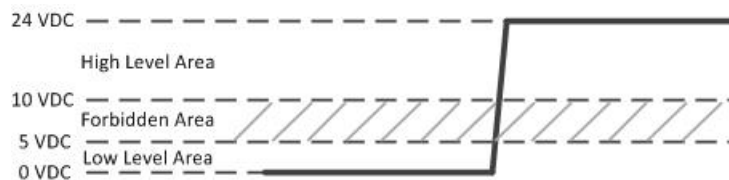
Figure 3-6: A Rising-edge Trigger Signal on Input
